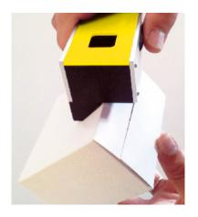
Our creasing measurement device CITO CREASY enables you to monitor creasing characteristics. It supports you during setup on the press, resulting in superior creasing and a longer service life for your tooling and creasing matrices.
