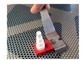
The magnets hold the telescopic presser extremely tight on the perforated plate. This connection can be easily released using a special lifter. The T-nut here acts as the anchor in which the lifter engages.
