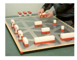
With the further improved blank'fix+, the separating blocks of differing size are simply positioned on a special galvanized and perforated plate and firmly anchored there using super-strong magnets.
